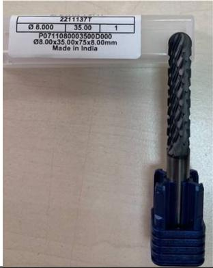
A photograph of a blue end mill with a silver cutting edge. The label above it reads: 2211137Y, Ø 8.000, 35.00, 1, P0711080003500D000, Ø8.00x35.00x75x8.00mm, Made in India.                  |
