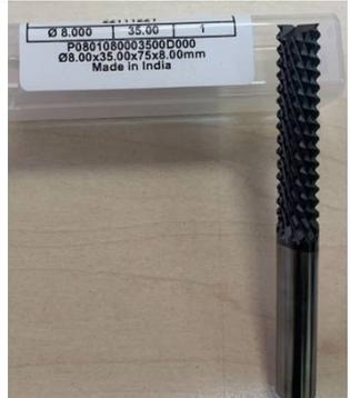
A photograph of a black end mill with a diamond coating. The label on the packaging reads: CONTOUR RTR M P0801, 22111231, Ø 8.000 35.00 1, P0801080003500D000, Ø8.00x35.00x75x8.00mm, Made in India. |
