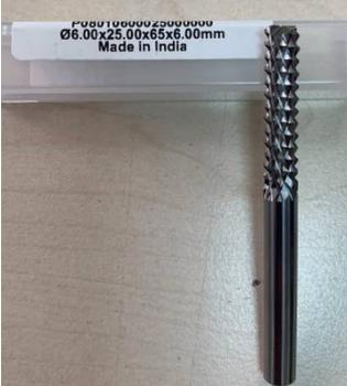
A photograph of a silver end mill without a coating. The label on the packaging reads: CONTOUR RTR M P0801, 22111231, Ø 6.000 25.00 1, P08010600025000000, Ø6.00x25.00x65x6.00mm, Made in India.    |
