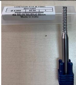
A photograph of a silver end mill without a coating. The label on the packaging reads: CONTOUR RTR M P0801, 22111231, Ø 4.000 20.00 1, P08010400020000000, Ø4.00x20.00x60x6.00mm, Made in India.    |
