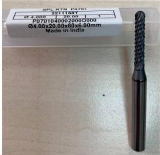
A photograph of a blue end mill with a silver cutting edge. The label above it reads: SPL RTR P0701, 2211138Y, Ø 4.000, 20.00, 1, P0701040002000D000, Ø4.00x20.00x60x6.00mm, Made in India.   |
