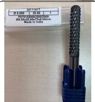
A photograph of a blue end mill with a silver cutting edge. The label above it reads: 2211141Y, Ø 8.000, 35.00, 1, P0701080003500D000, Ø8.00x35.00x75x8.00mm, Made in India.                |
